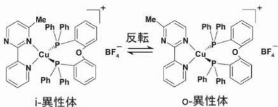
Figure 2 Two isomers of [\text{Cu}(\text{Mepypm})(\text{DPEphos})]\text{BF}_4 ( 1\cdot\text{BF}_4 ) and interconversion with pyrimidine ring rotation.
