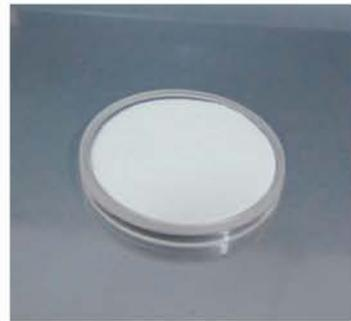
Figure 1 Snapshot of the SVOC sampler.
